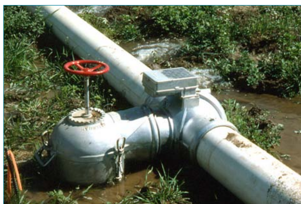
Figure 2. A controller on the surge valve allows the grower to manage the duration of the wetting and soaking cycles.
