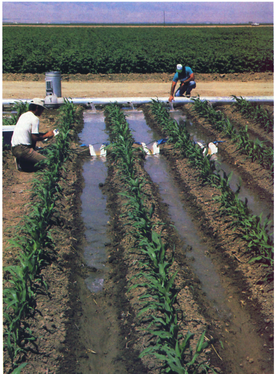
Surge irrigation, in which water is released into furrows intermittently instead of as a continuous flow, may reduce irrigation water needs by a third, substantially reducing drainage requirements. UC researcher Dave Goldhamer (top) and visiting Japanese scientist Tomoo Inaba check the flow of water from the main feeder line through RBC flumes that measure in-furrow flow rates.
