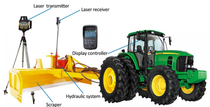
Figure 3. Example of laser land leveling system ( http://www.shtbag.com/productsInfoEng.html ).
